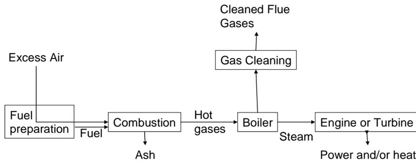
Figure 6. Flow chart of a conventional combustion system (based on Figure 2 in (Schuck, 2006)).
