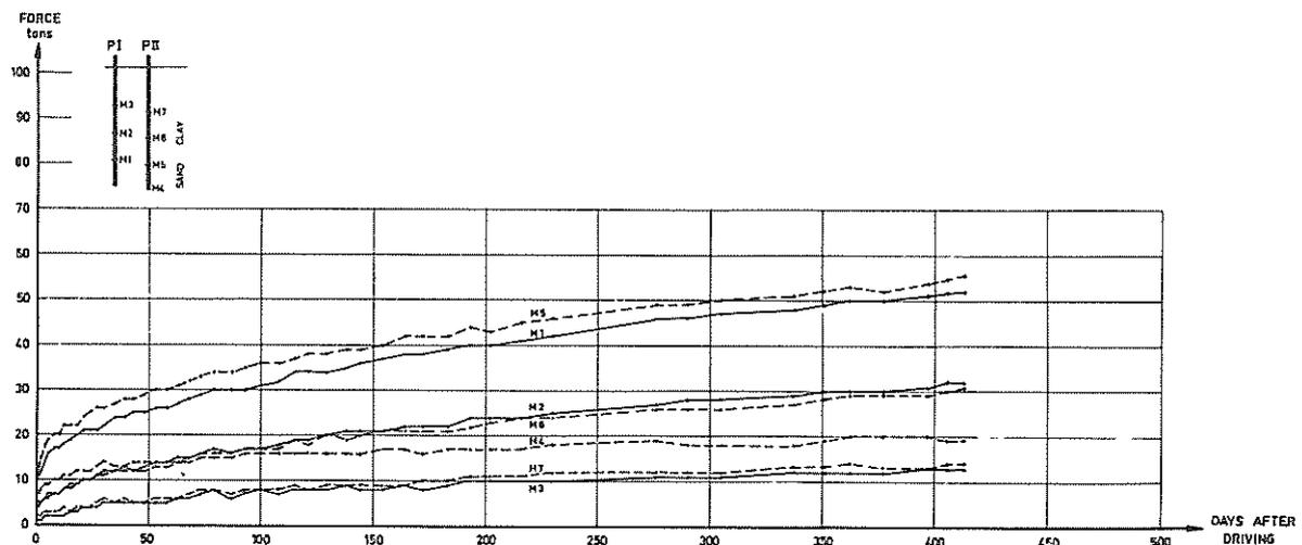
Fig. 1 Recorded loads in piles P I and P II
