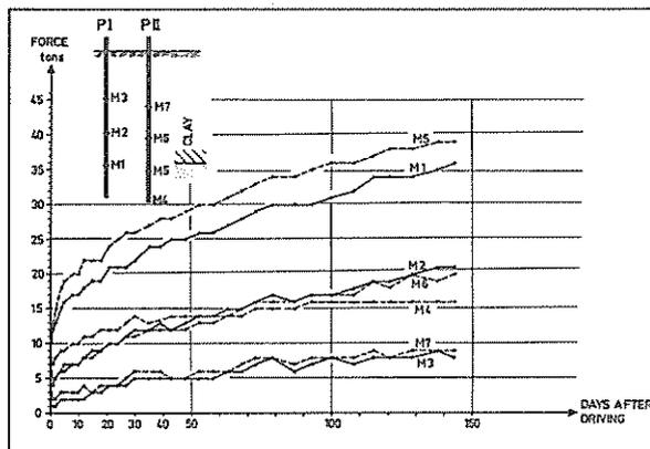
Fig. 6 Recorded forces in piles PI and PII
