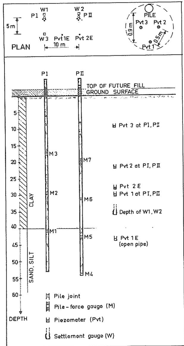
Fig. 3 Location of piles and instrumentation
